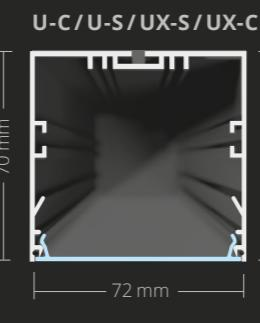
The variability of U PROFILES allows U-luminaires to be installed either as a recessed (U-T framed or U-R trim-less version), ceiling-mounted (U-C; UX-C) or suspended (U-S; UX-S)
